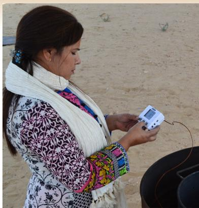
*During biochar production temperature was controlled through a thermocouple.*
