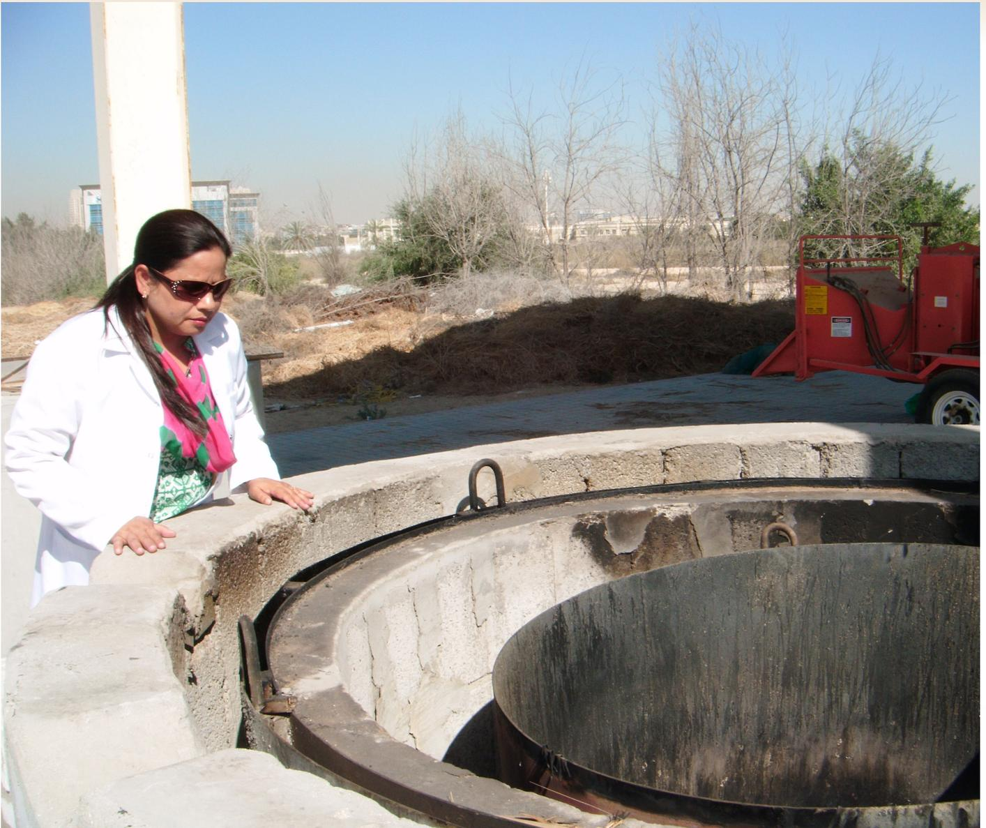
An on-farm biochar production facility at the ICBA station. Biochar is produced through recycling date palm feedstock collected from the experimental station.
