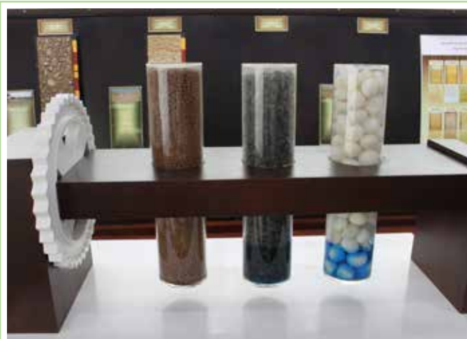
The Water Infiltration Simulation Unit demonstrates how sizes of soil particles (sand, silt, clay) in soil influence infiltration rate.
